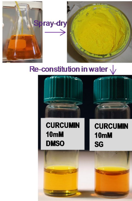
Figure 1. SG-solubilized curcumin in water solution can be spray-dried to SG-encapsulated powder and completely reconstituted in water. To make a 10 mM stock solution of curcumin, 16% w/v SG is needed compared to the same 10 mM stock by absolute DMSO.
